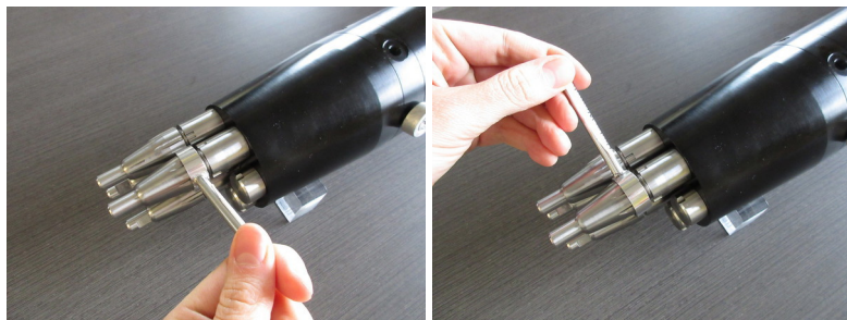
Figure 9: Loosening the probe holder using the custom probe wrench.
