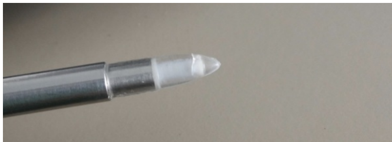
Figure 37: A shear probe with a crack in the silicone tip.
