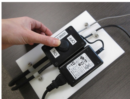
Figure 29: Sending the ON signal using the deck unit switch.
