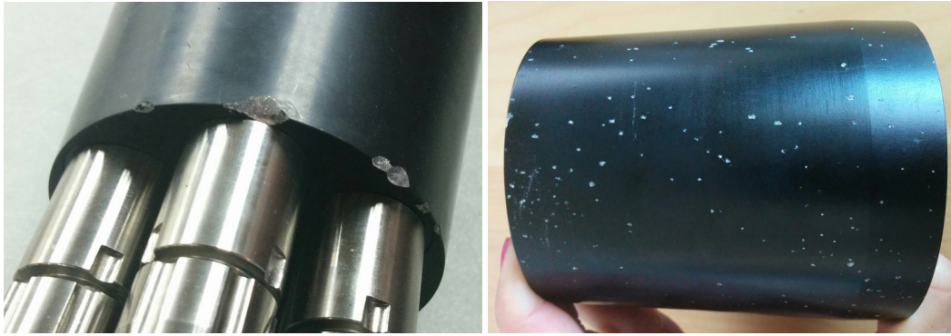
Figure 34: Extreme corrosion on a MicroRider1000 after a long-term deployment
