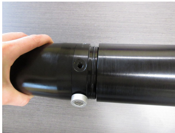
Figure 18: Separating the front bulkhead from the pressure tube.
