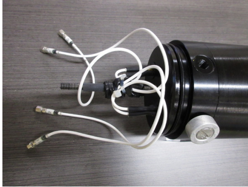
Figure 22: Nose cone removed, revealing the SMC cables and the threaded rod.
