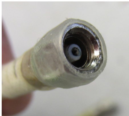
Figure 35: Green corrosion on the inside pin of an SMC connector. Without corrosion, the pin would appear shiny and gold.
