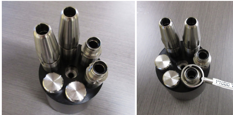
Figure 23: Removal of the probe holders from the nose cone.
