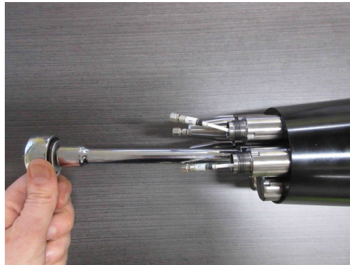
Figure 21: Loosening the front sealing nut with a socket wrench (with extension).
