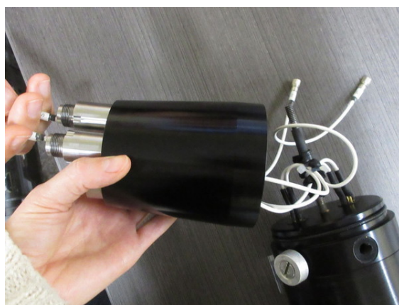
Figure 24: Feeding the SMC cables through the nose cone. The picture shows the probe holders already installed on the nose cone. It is recommended that you first install the nose cone, and then install the probe holders.
