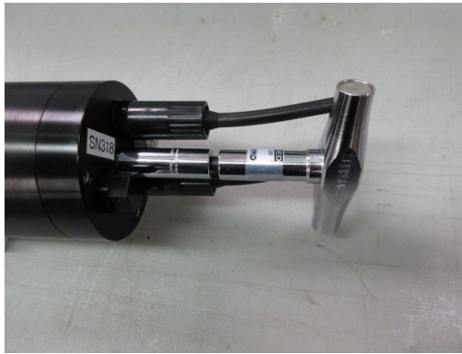
Figure 15: Removing the sealing nut.
