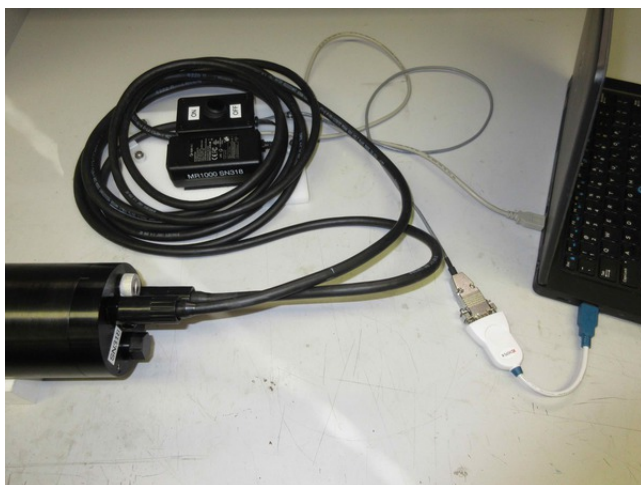
Figure 31: Connecting the deck cable to the computer.
