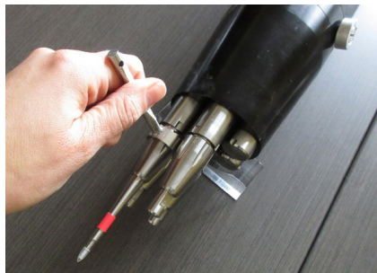
Figure 12: Tightening the probe holder.
