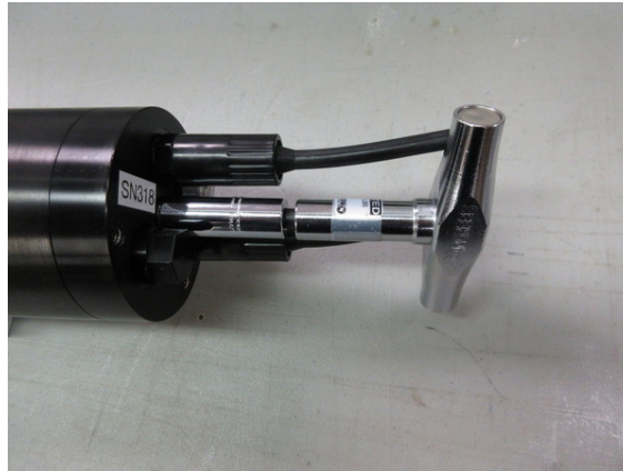
Figure 28: Tightening the sealing nut on the rear bulkhead.
