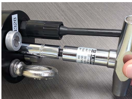
Figure 16: Removing the sealing nut
