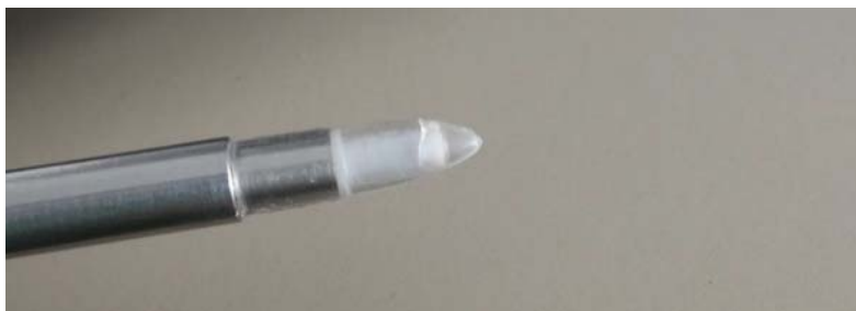
Figure 42: A shear probe with a crack in the silicone tip.
