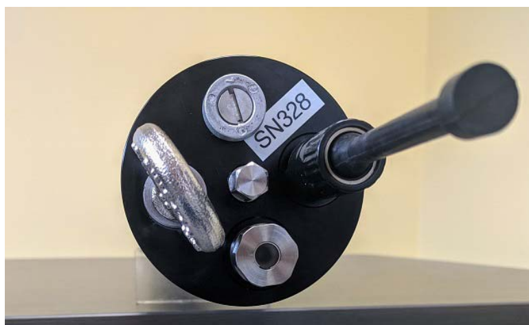
Figure 19: VMP-250-IR Rear Bulkhead. Note the lifting ring is rotated such that it is entirely within the diameter of the instrument. The lifting eye orientation can be adjusted using washers as shims.
