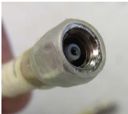
Figure 40: Green corrosion on the inside pin of an SMC connector. Without corrosion, the pin would appear shiny and gold.
