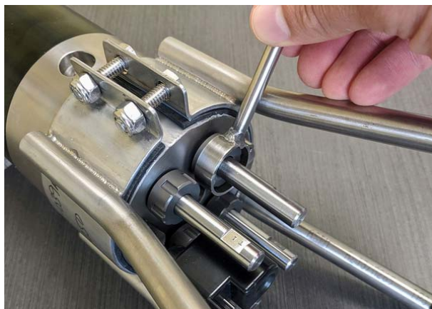
Figure 22: Loosening the probe holder using the custom probe wrench.
