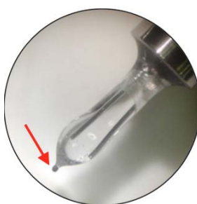
Figure 43: FP07 thermistor. The small sensing tip is indicated by the red arrow.
