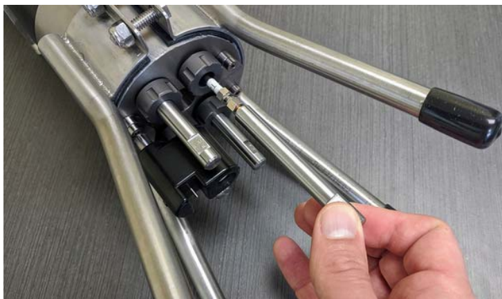
Figure 23: Removing the test probe. Note the clear heat shrink tubing around the SMC connector.
