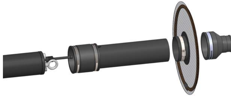
Figure 13: Assembling the drag net and rubber coupler onto the tail section.
