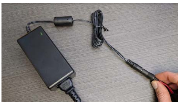
Figure 34: Connecting the AC adapter cable to the Deck Cable
