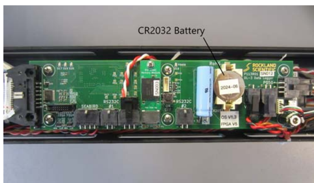
Figure 10: CR2032 Battery on Rockland Data Logger board
