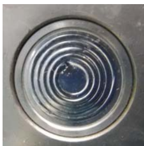
Figure 44: A dent visible on the thin diaphragm of a PA10L pressure sensor
