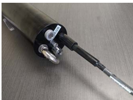
Figure 27: Connecting the deck cable to the instrument.
