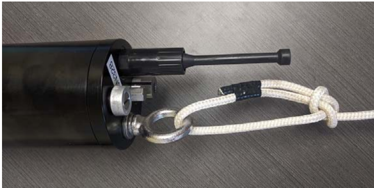
Figure 14: Tether tied and secured to the instrument with a bowline. Note: Tail section not shown for clarity.
