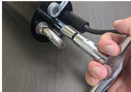
Figure 20: Tightening the Sealing Nut
