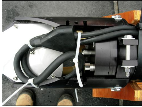
Figure 24: Typical SBE3/4 Cable routing.
