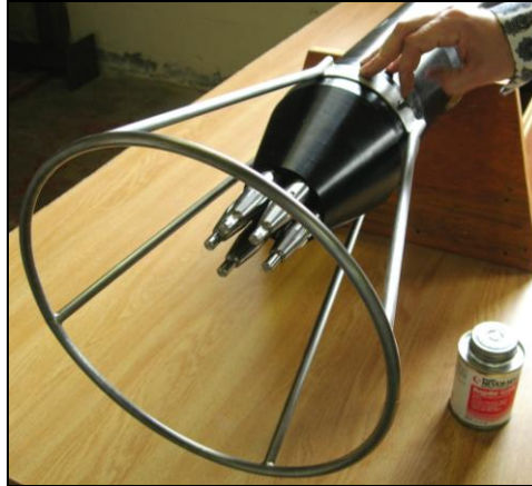
Figure 6: Installing bolts with Never-Seeze on threads.
