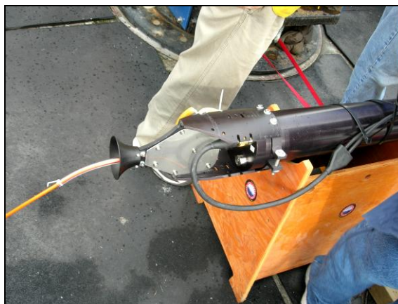
Figure 20: Tether clamp plate installed
