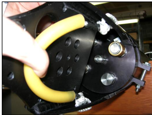
Figure 9: Groove-less side of Tail Fin aligned with Tether “T” connector.
