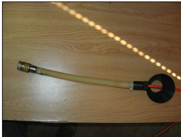
Figure 15: Tether Cable routed through bellmouth.
