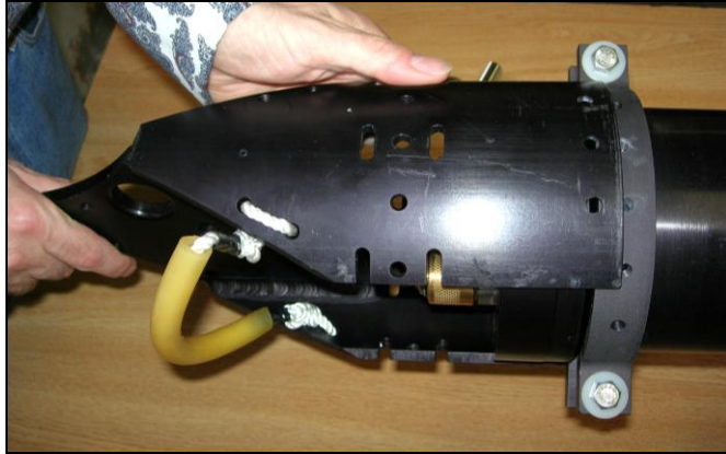
Figure 8: Sliding Tail Fin over Rear Bulkhead/Mounting Clamps.
