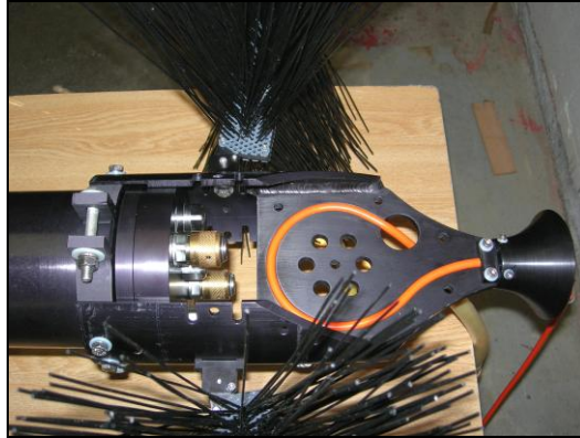
Figure 18: Cable in groove and funnel mounted to tail fin
