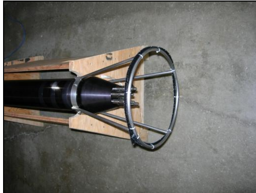
Figure 4: Eddy Shedding Brush on Guard Ring.
