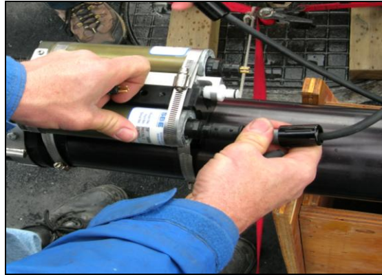
Figure 21: Connecting SBE3/4 Cables.
