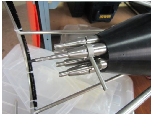
Figure 32: Probe Seated and Holder Tightened.
