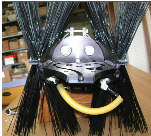
Figure 12: Brushes installed 180° to each other.
