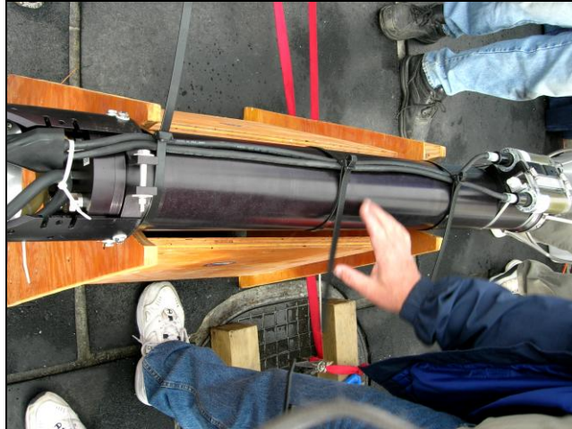
Figure 22: SBE3/4 Cable secured to Pressure Tube.
