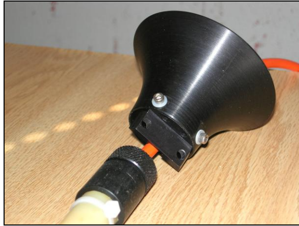
Figure 16: Funnel bracket attached to bellmouth.
