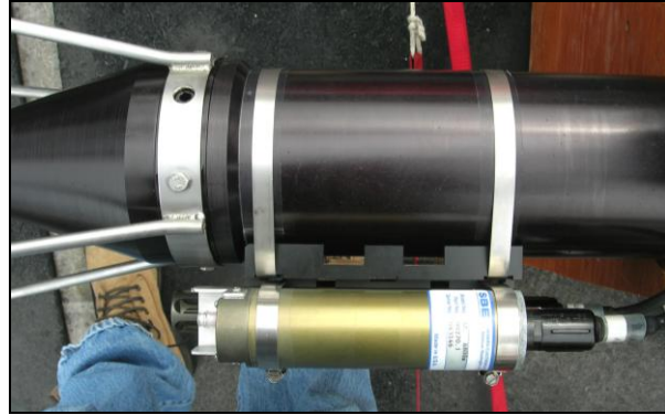
Figure 14: Mounted SBE3/4 Bracket Assembly.
